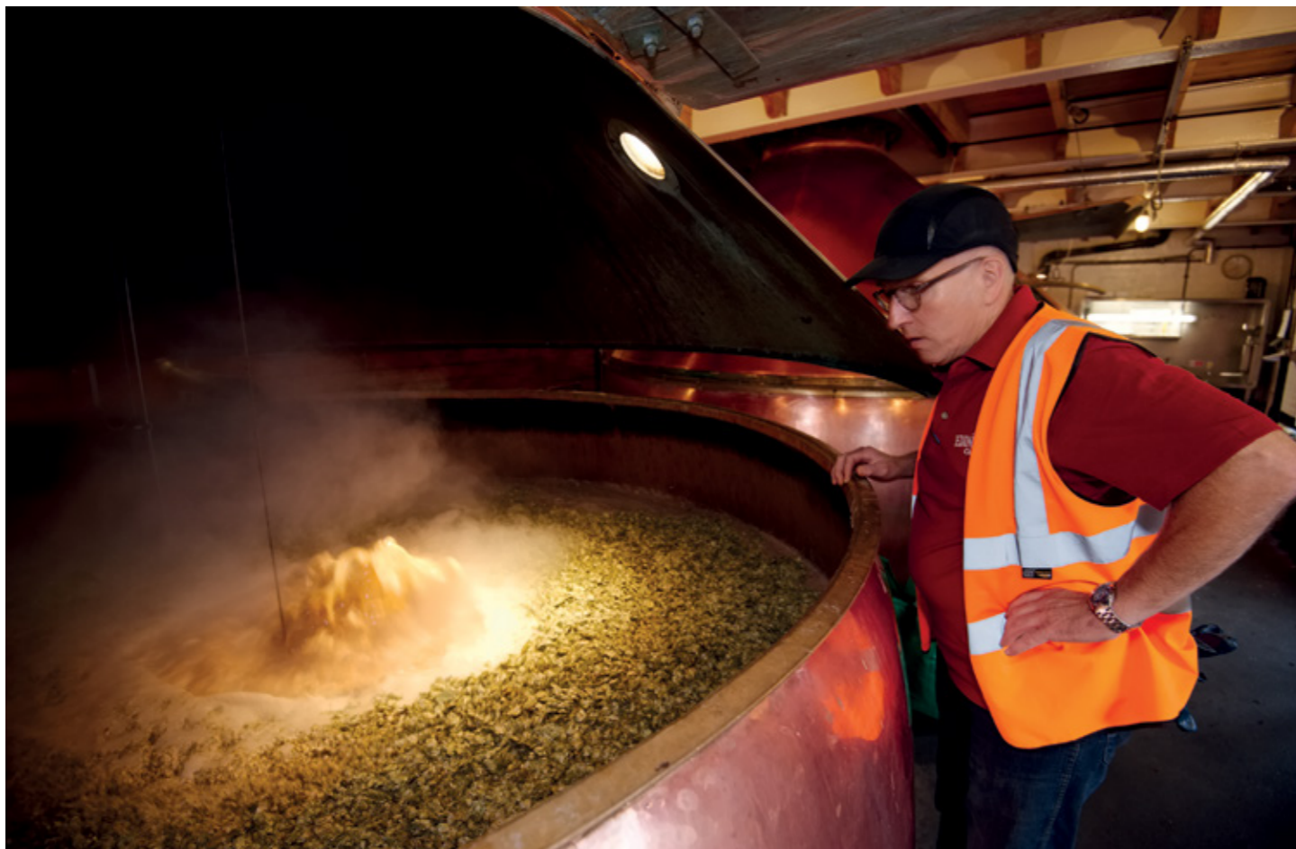
Open fired copper kettle at The Caledonian Brewery boils beer wort and hops.
